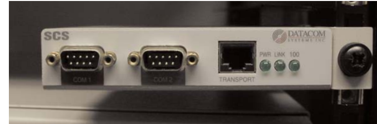
SCS fastened on the right side of the equipment rack
