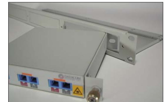
Put FIBERTap™ through knockout opening
