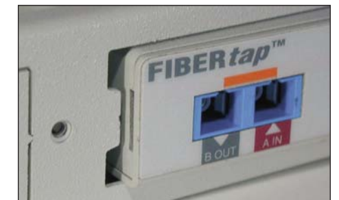
Align knockout tab and FIBERTap™ slot
